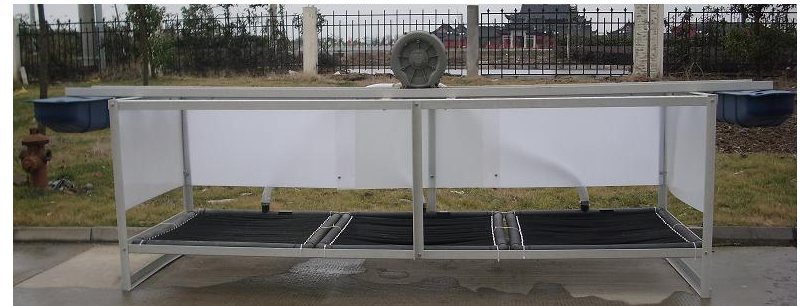
3 Grid Airlift Model, simple construction using non corrosive, light fibreglass frame & 3 airlift grids
